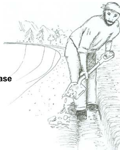
Step 4 Excavate a 300 x 300 anchor trench around the perimeter
