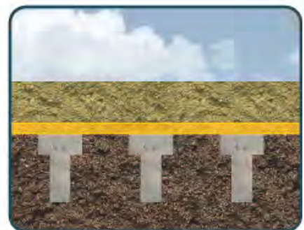
Basal reinforcement over piled foundations
