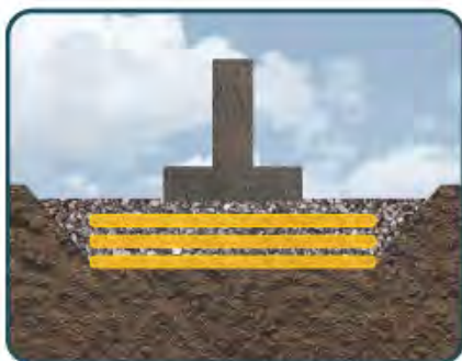
Foundation cushioning, soil stabilisation
