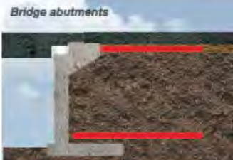
Base course reinforcement
