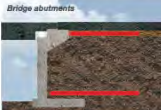
Base course reinforcement
