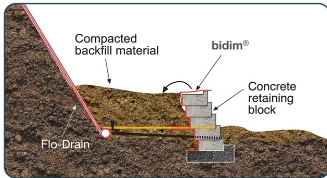
Outlet pipes from the cut-off drain through the engineered fill and wall face discharge water in a controlled manner to existing stormwater systems.
