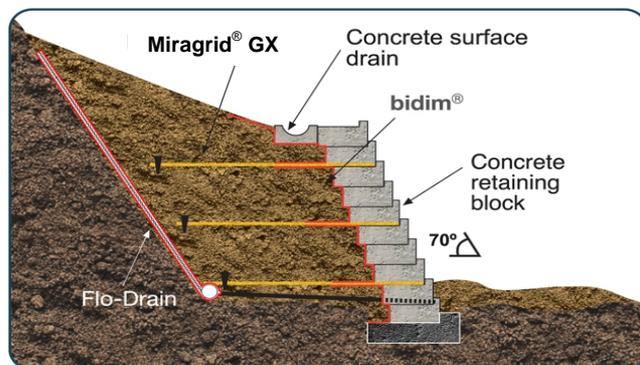
Continue with steps 5, 6 and 7 until the height of where the reinforcement needs to be placed is reached. The geogrid reinforcement needs to be installed progressively within the engineered fill as construction of the block wall proceeds.
