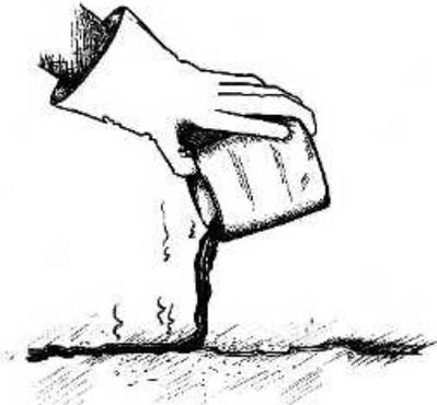
2. Prefill larger cracks (wider than 7mm) with a 0.5mm crusher dust 5.3ℓ, cement 0.25ℓ, latex modified cationic emulsion 2ℓ and water 1ℓ mix.
