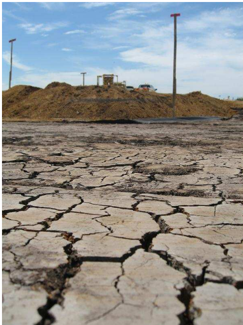
Left: Typical ground condition, alluvial crust overlying very soft clay and peat
