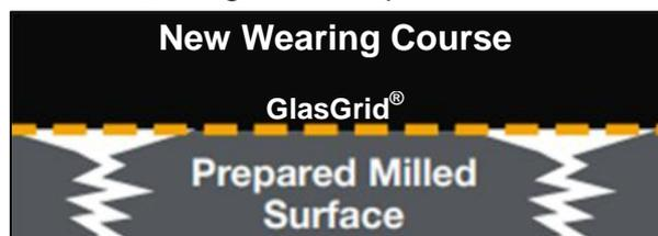
This 50 kN x 50 kN tensile strength, glass reinforced geogrid is designed to redirect crack stresses horizontally and dissipate traffic induced stresses.
